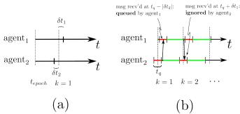
Figure 5: Here, agent<sub>1</sub> is delayed relative to the ground truth clock  $(\delta t_1)$ ; agent<sub>2</sub> is ahead of time  $(\delta t_2)$ , (a). In (b), timebounded out-of-sync messages are dealt with by adding a quiescent period  $t_q$  (red), during which messages may be received, but are not sent. Messages with old timestamps are ignored within the quiescent period; successive rounds are indicated by k.
