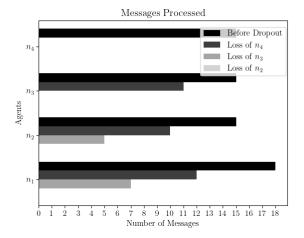
Figure 6: Messages processed by each agent after successive reelection cycles following the loss of an agent in  $\mathcal{G}$ . Note that this demonstration includes additional message counts for a Convergecast of each child in LeaderSelection.
