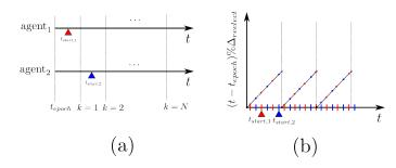
Figure 4: Agent queries are performed assuming a hardwaredriven periodic timer. Agents desire reelection at every kth reelection interval (a), but agents might start ahead of or behind the ground truth clock. Regardless, queries can be made at the timer frequency f, providing a trigger if the k-th reelection period has been passed, (b).
