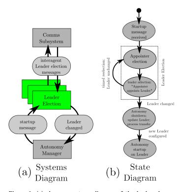
Figure 2: (a) shows a systems diagram of the leader election process on each agent (green) which communicates with a message-passing layer (comms) to pass messages between agents and convey a leader to an autonomy manager. (b) shows state transistions of each leader election process synchronizing an initial election round, followed by persistent reelection cycles following Figure 3. A leader change restarts leader-dependent processes on each agent, such as those of an autonomy manager.
